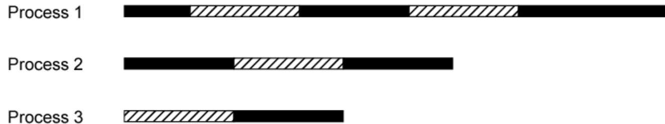
(b) Interleaving and overlapping (multiprocessing; multiple processors)
