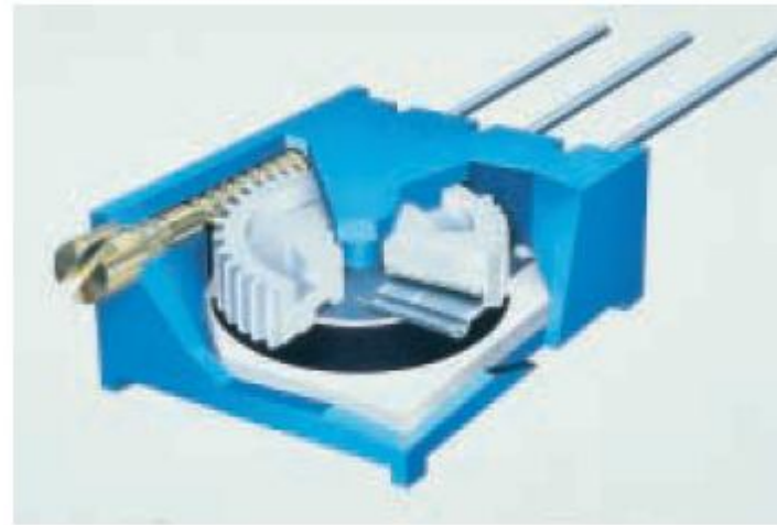
(b) Internal view of variable resistor.
