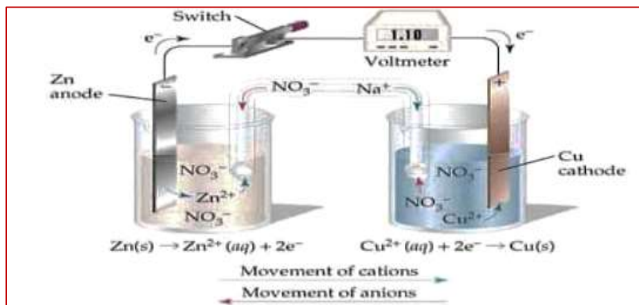
Figure 1: Functioning of a Daniell cell (Zn-Cu) using a salt bridge
